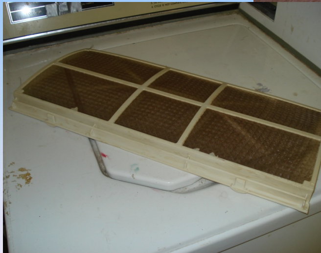
A/C Filter With Smoke Damage
