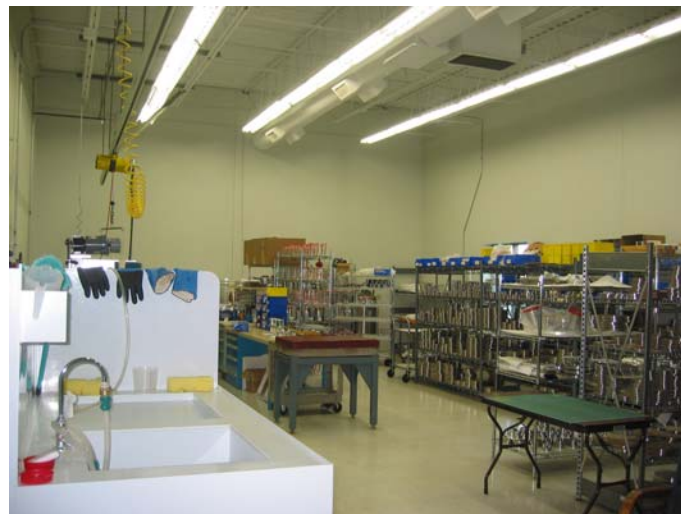
Packaging Clean Room (Class 10,000 with Positive Pressure)
